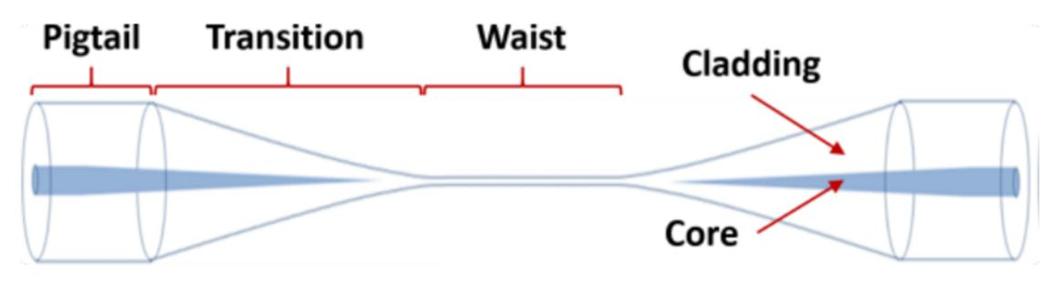
The "pigtail" has the dimensions of a normal optical fiber. It has a radius of about  $10^{-3}m$ . However, the "waist" of the optical nanofiber is about  $10^{-6}m$ . The cladding material guides the light as it is transmitted through the "core" of the fiber.
