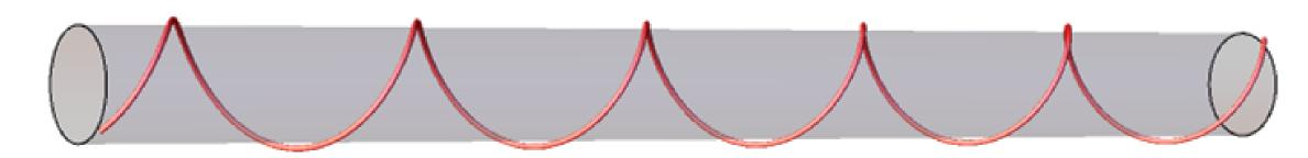
The red tube is the trajectory of the particle and the cylinder represents the waist of the nanofiber. As the particle traverses this trajectory, it spins rapidly. Our analysis also showed that the period of the spin of the particle is small ( $\approx 10^{-2}$ s) compared to the period of revolution ( $\approx 10^{6}$ s) around the nanofiber. So the particle spins about one of its axis many times before it orbits the fiber once.
