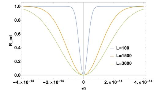
Rate of coincidences for BBO crystal at  $\alpha = 1.0615$  for 3 different lengths
