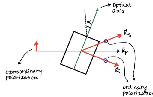
Process of spontaneous parametric down conversion, one extraordinarily polarized photon passing through birefringent crystal
