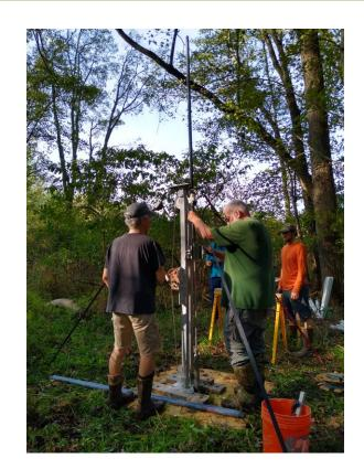
In the field, we extracted a 1-m sediment core near the lakefront using a modified-Livingstone sampler. The core contains diatoms, mostly from pre-settlement and post-settlement times. We also sampled the lake's sediment-water interface using a probing instrument to collect modern diatoms.
