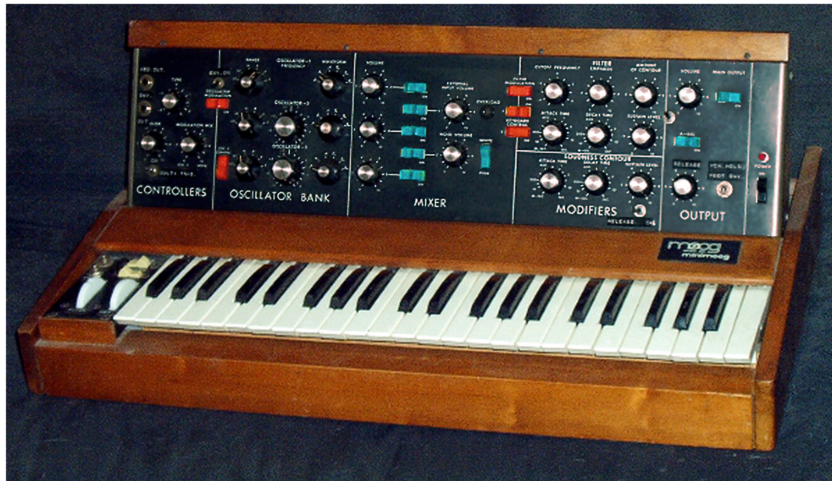
Figure 1. The Minimoog Model D. An influential modular synthesizer, this is the first commercial modular synthesizer which contains several fundamental synthesizer concepts found today.
