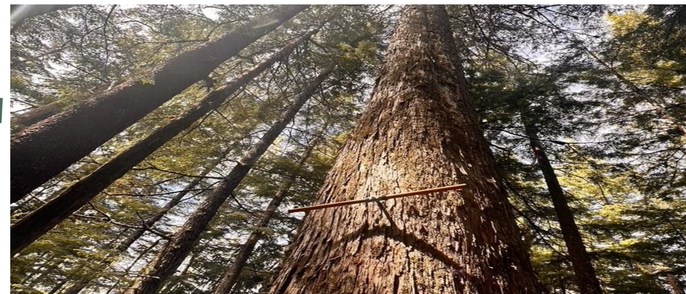
Figure 5 - A increment borer in a yellow cedar in SE Alaska collecting a tree ring core.
