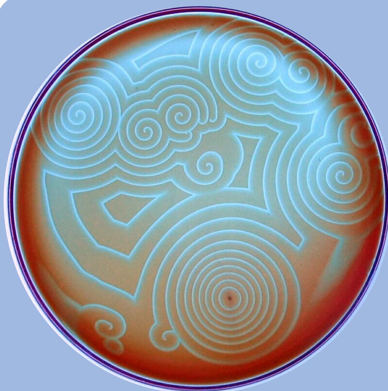
Fig. 1: Example of several BZ waves and spirals propagating in a Petri dish [3].
