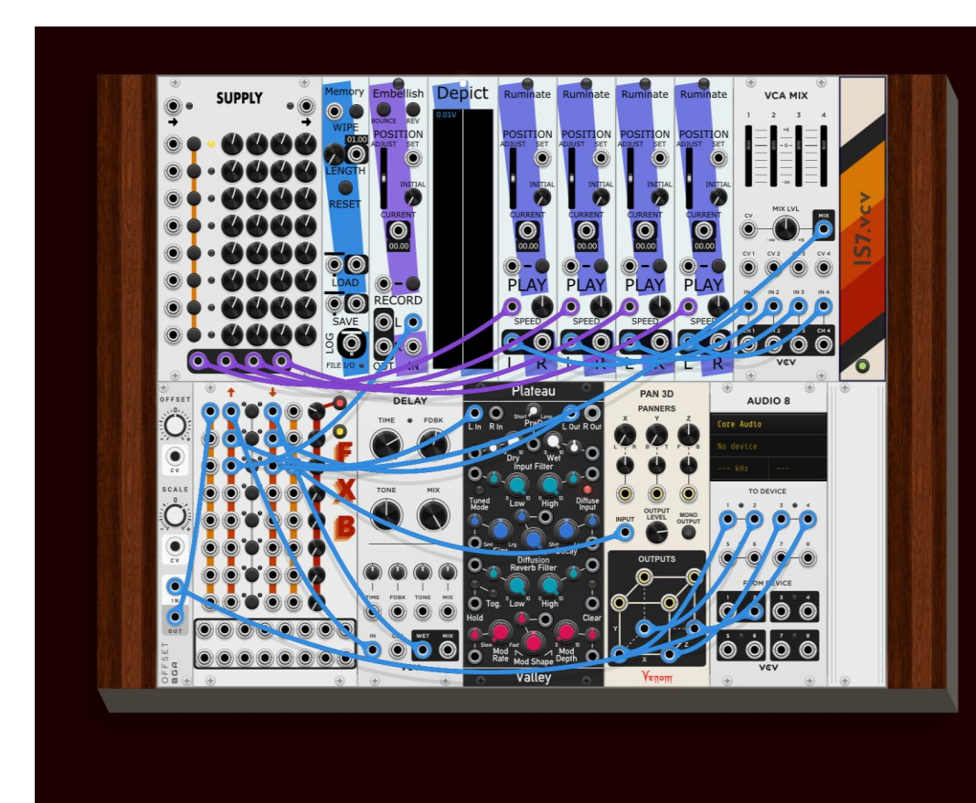
Up: A basic synthesizer voice assembled in VCV Rack
