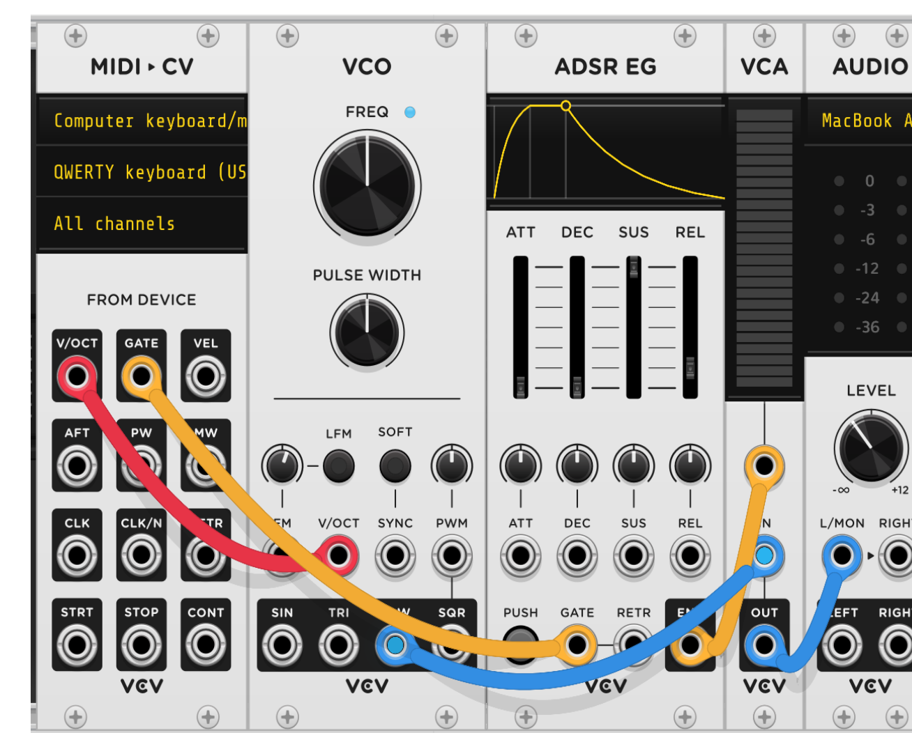
Up: A basic synthesizer voice assembled in VCV Rack
