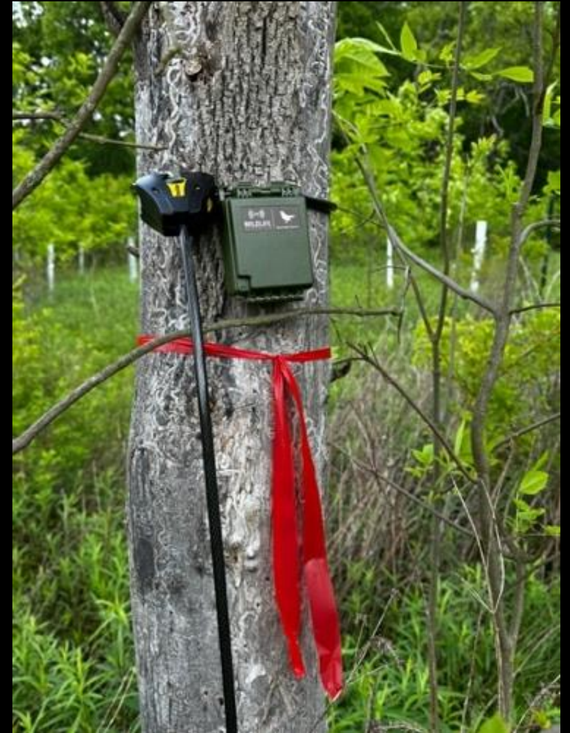
Figure 2: Tree where a bioacoustic recorder was placed. The recorder was secured using a locking cable tie, and flagging tape was tied to the tree for visibility purposes.
